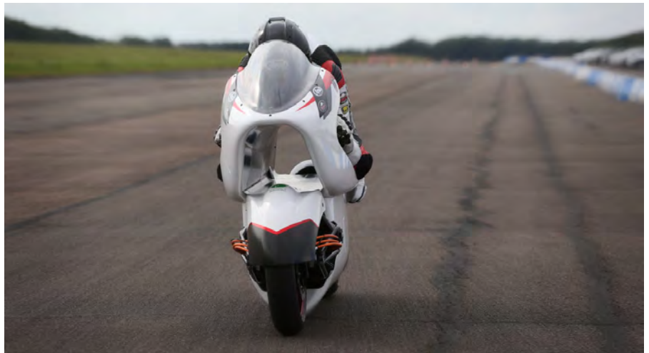
Figure 1: WMC250EV aerodynamic assessment – track testing
